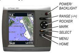
**POWER/BACKLIGHT**—Press and hold to turn the unit on or off. Press and release to adjust the backlight and the day and night modes.
